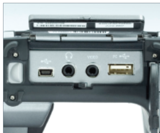
From Left to right: USB mini for PC image download, 4 pole audio for voice annotation, NTSC video, USB-A for memory stick image transfer
