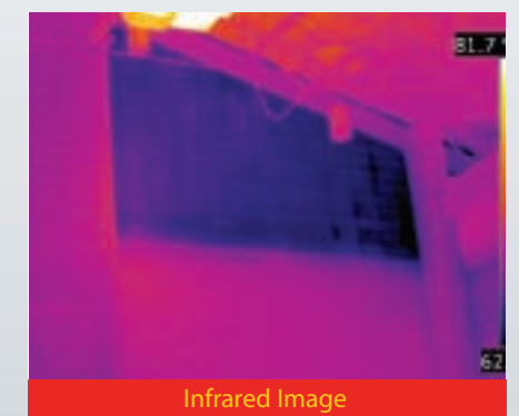
Fusion Image Showing Missing Insulation
