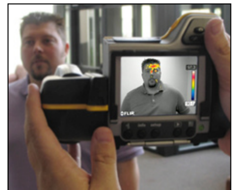
Handheld T360 with “threshold fusion” and “color alarming” in visible camera mode.
